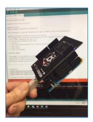
NeuroShield SPI connectivity is directly compatible the Arduino UNO, Duemilanove and 101.
