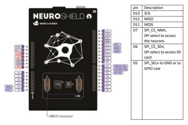
If using the USB port for power supply, do not forget to connect a GND pin of the NeuroShield to a GND pin of the host.
